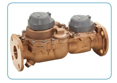
Rotor and disc movements are transmitted by magnetic drive couplings to individual register odometers. The direct magnetic drive provides a positive, reliable and dependable register coupling for straight-reading or remote reading options. The self-lubricating thermoplastic register gearing is designed to minimize friction and provide long life.
